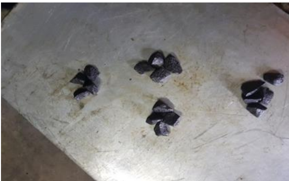
Photos 9 (a), (b), (c) and (d) - Continuing the process of coning and quartering
