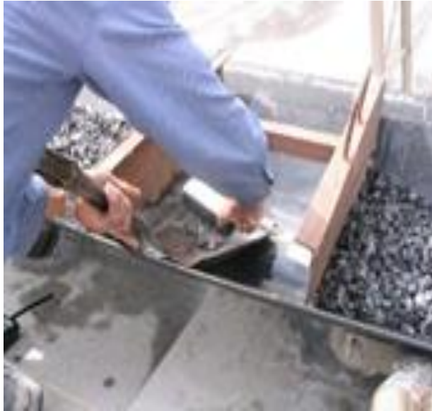
Brushing all fines remaining on conveyor belt
