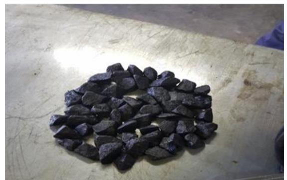
Photo 6 - Pressing the coned material flat
