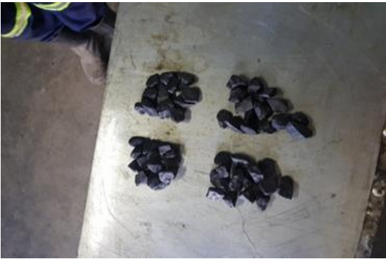
Photo 7 - Dividing material into four quadrants
