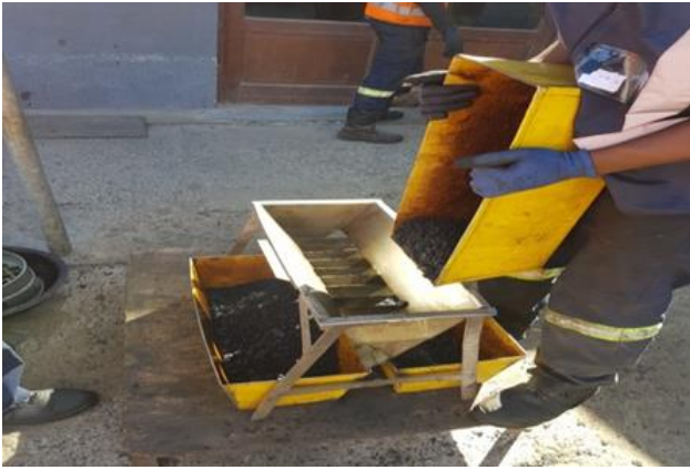
Photo 1 - Splitting the material in two equal halves
