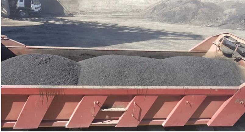
Figure A3: Typically Loaded Asphalt Delivery Vehicle (Three Piles from the Asphalt load-out hopper)
