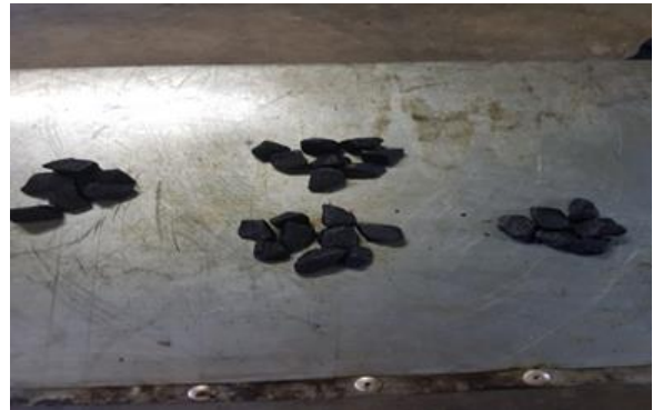
Photo 8 - Rejecting the two opposite quadrants
