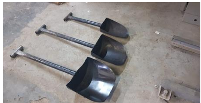
Figure A2: Large, Medium and Small Scoop Shovels
