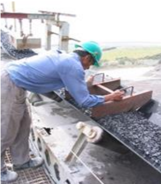
Sampling templates placed in position on halted conveyor belt
