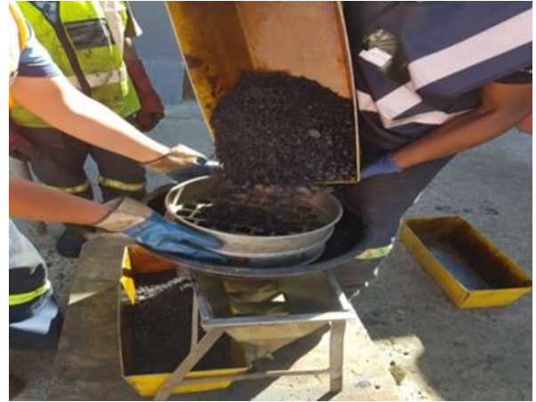
Photo 2 - Sieving extra-large particles
