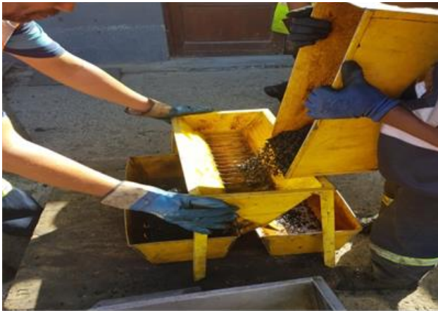
Photo 3 - Second splitting procedure
