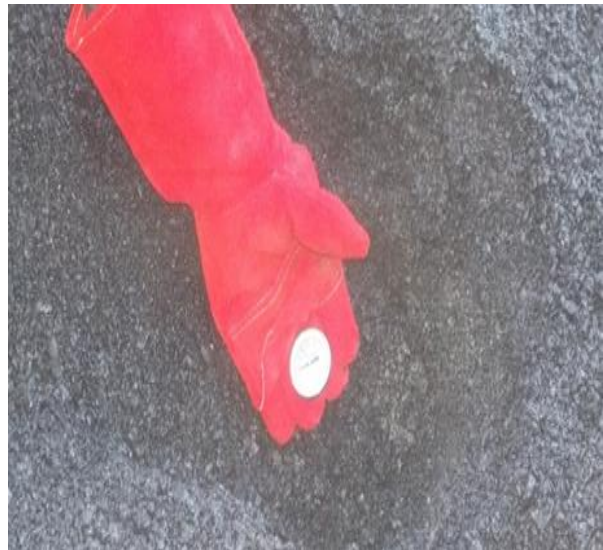
Figure A5: Dial-Gauge Temperature Device in Sample Hole
